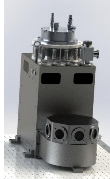
Commercial closed-cycle optical access cryostat: OptiDry from MyCryoFirm
