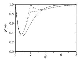
Fig. 12. Fraction  $\Phi''/\Phi'$  of the flux remaining after the second antenna as a function of its parameter  $\eta_2$ . The first antenna is driven at a frequency  $\nu_1 = \eta_1 k_B T/h$  with  $\eta_1 = 2 = 1.6 \eta^*$ . The dashed line corresponds to the collisionless regime; the dotted line to a mean number of collisions between antennas  $N_c = 1.1$ ; the solid line to full rethermalization. These curves are calculated with a numerical simulation, in the case of a linear confinement.
