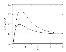
Fig. 9. Gain in phase space density after evaporation by one antenna and rethermalization, as a function of  $\eta$ , for the multiradii evaporation scheme. Solid line: harmonic confinement; dashed line: linear confinement.
