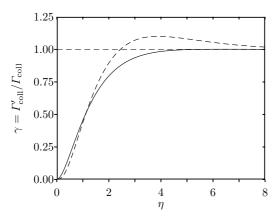
Fig. 10. Variation of the collision rate after evaporation by one antenna and rethermalization, as a function of  $\eta$ , for the multiradii evaporation scheme. Solid line: harmonic confinement; dashed line: linear confinement.
