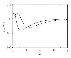
Fig. 4. Temperature change  $\tau = T'/T$  after evaporation by one antenna and rethermalization, as a function of  $\eta$ . Solid line: harmonic confinement; dashed line: linear confinement.
