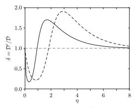
Fig. 5. Gain in phase-space density  $\mathcal{D}'/\mathcal{D}$  after evaporation by one antenna and rethermalization, as a function of  $\eta$ . Solid line: harmonic confinement; dashed line: linear confinement.
