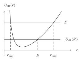
**Fig. 1.** Effective potential  $U_{\rm eff}(r)$ . An atom with  $E \geqslant U_{\rm eff}(R)$  is evaporated.
