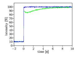
FIG. 5. (Color online) Time dependence of the laser intensity when switching the rf power rapidly. Without the second frequency (green), it takes nearly 10 s for the intensity to stabilize to its steady state value. With the second frequency (blue), there is only a very small transient effect during the first second after switching.
