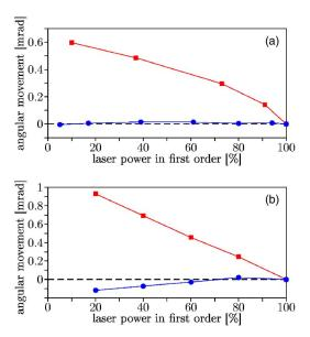
FIG. 4. (Color online) (a) Measured angular movement of the first order beam perpendicular to the plane of diffraction (y) with (blue circles) and without the second frequency (red squares) for the  $TeO_2$  AOM. The movement is plotted as a function of the relative laser power in the first order with respect to its maximum value. (b) Same measurement for the Ge AOM, measured in the diffraction plane x.
