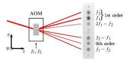
FIG. 3. (Color online) Schematic of the AOM driven by two frequencies. The image shows a picture of the laser beam diffracted by the  $TeO_2$  AOM. On the right hand side of the image, the frequency shifts corresponding to the diffracted light are indicated ( $f_1$ =99 MHz and  $f_2$ =123 MHz).
