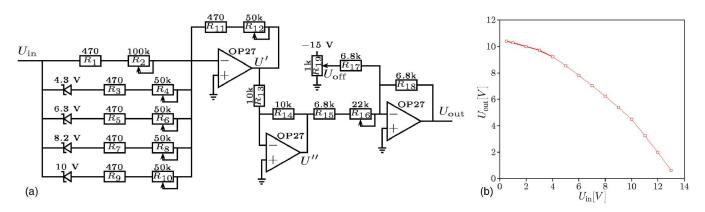
FIG. 6. (Color online) (a) Schematic of the electronic circuit for adjusting the control voltage. The gain of the first inverting amplifier depends on the voltage  $U_{\rm in}$  due to the Zener diodes. The amplified voltage is inverted again before a variable offset  $U_{\rm off}$  is added in the last step. (b) Measured transfer function of the circuit
